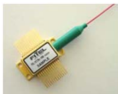
The high-output narrow-linewidth full-band tunable laser
